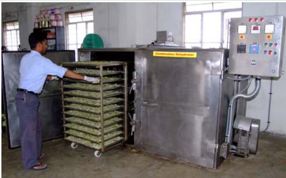
Perforated trays with Kokum loaded in a hot air dryer
